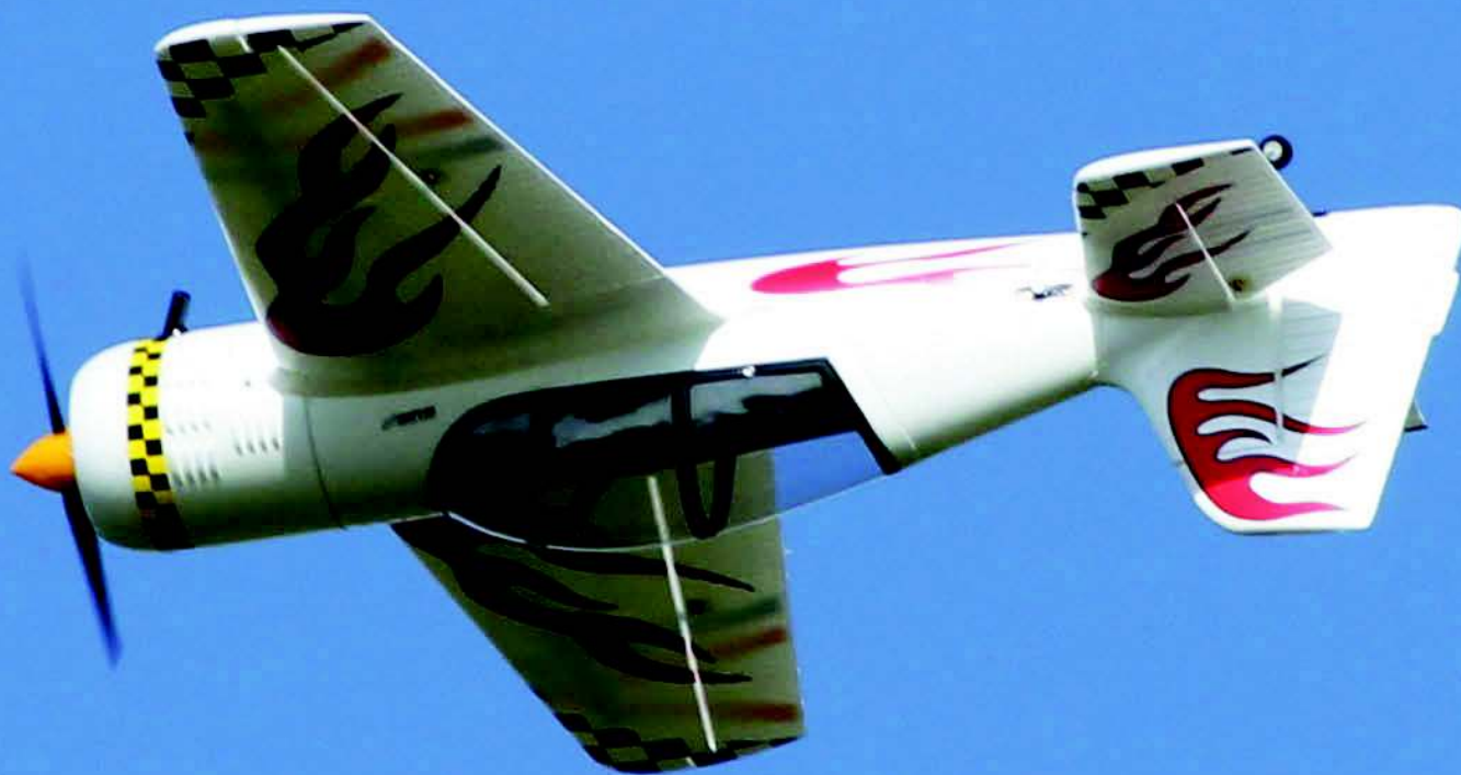
Inverted flight only needs a dab of down elevator
