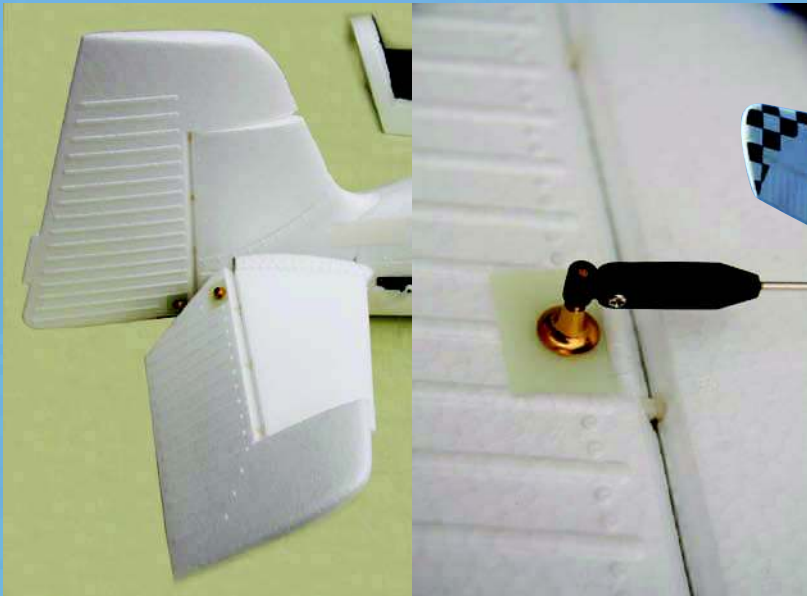
Horizontal and vertical stabilisers in place
