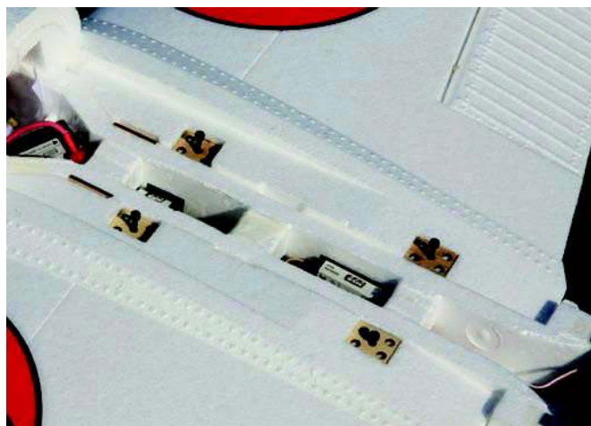
Wings aligned and held in place by four cap-head screws
