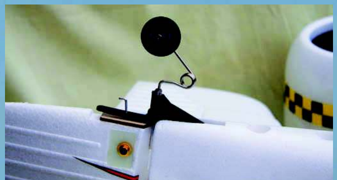
Tail wheel is bolted to fuselage and steering provided by pin on rudder
