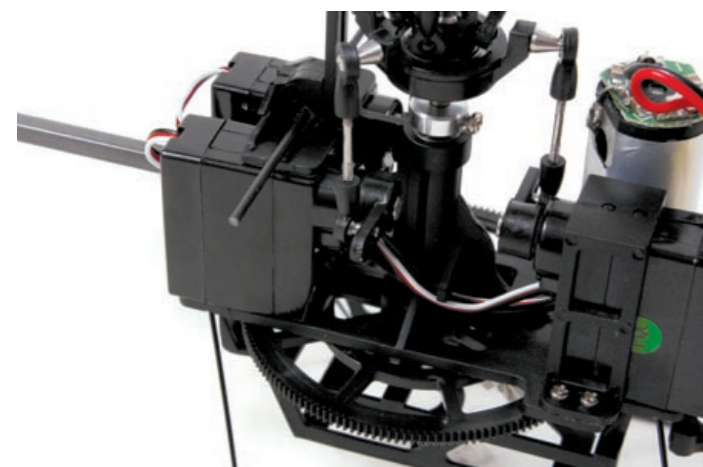
The servos are tiny, but are proper separate units, not surface mounted
