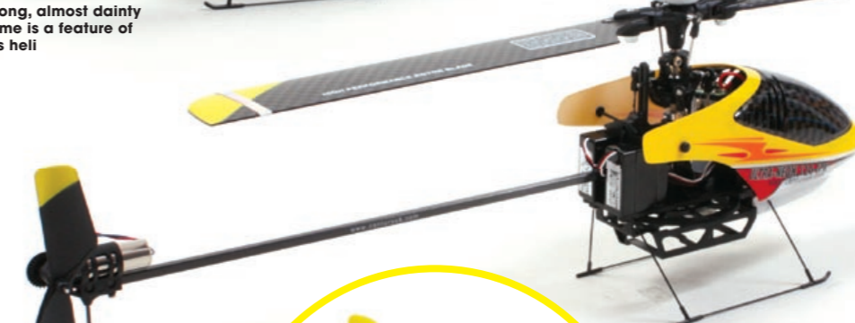
Whilst the main rotor head is driven by a larger brushed motor under the canopy
