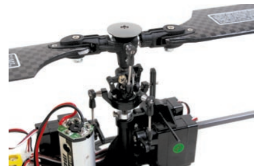
The flybarless head is plastic, but very well engineered. The top button is however, aluminium
