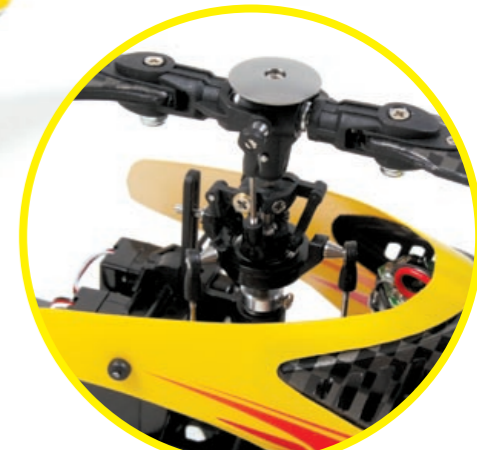
Whilst the main rotor head is driven by a larger brushed motor under the canopy
