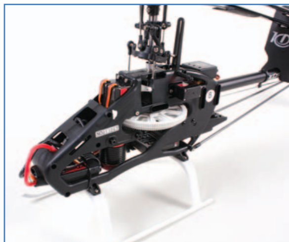
The plastic frame is a complex and stiff moulding that gives a solid mounting for all the major components
