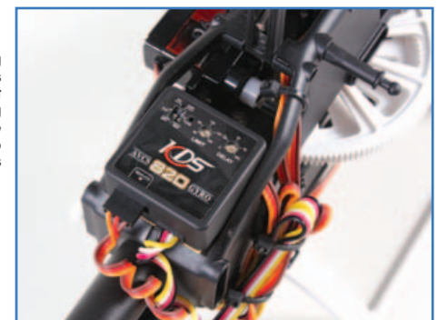
The heading hold gyro is strong and fast responding and can be adjusted to your tastes
