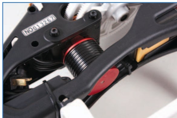
KDS' own outrunner brushless motor provides plenty of power yet runs cool
