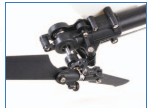
The tail gearbox and blades are again plastic
