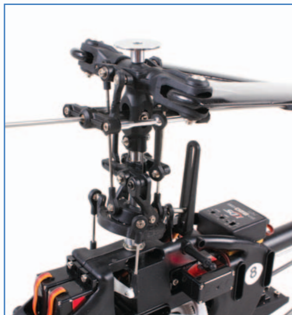
The head is plastic and features a fly-bar and 120 degree CCPM
